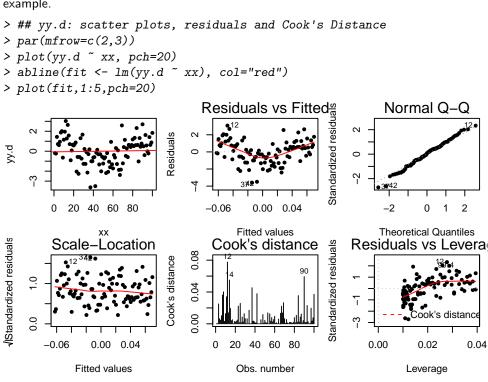
yy.d: In case of the fourth model, the systematic error can be easily detected in the Tukey-Anscombe plot since it exhibits a U-shaped pattern. The Normal plot and the scale-location plot do not show any abnormalities. There are no influential data points but the smoother deviates from the horizon in
