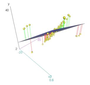
The 3D plot contradict the above conclusion. The majority of the data points scatters around a plane that is completly different from the OLS solution. Additionally, there are a few high leverage points that lies outside the point cloud on both sides of the regression plane. The OLS fit tries to accomodate all
