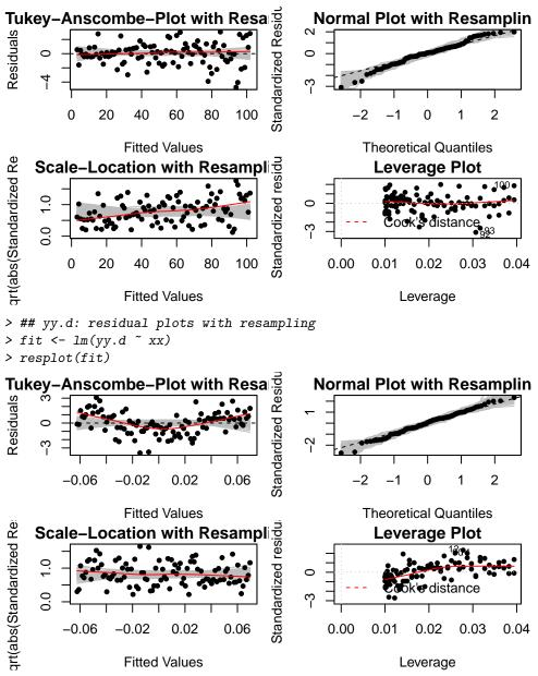
As you can see from the plots, the function does a good job in detecting the three model violations. Additionally, it does not make a mistake "in the other direction", either. I.e. the smoother does not lie outside of the gray area in cases where the model assumptions are fulfilled. In other words, there are no "false positives".
